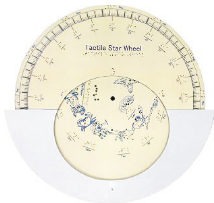
[Fig. 1] Proposed tactile star wheel
