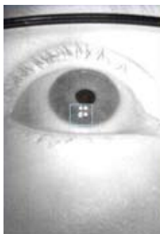
[Fig. 4] Cursor moves up – controlling by eye movement
